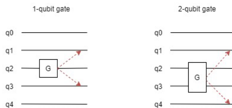
Figure 1: Crosstalk of gate G on neighbouring qubits for 1-qubit and 2-qubit gates
