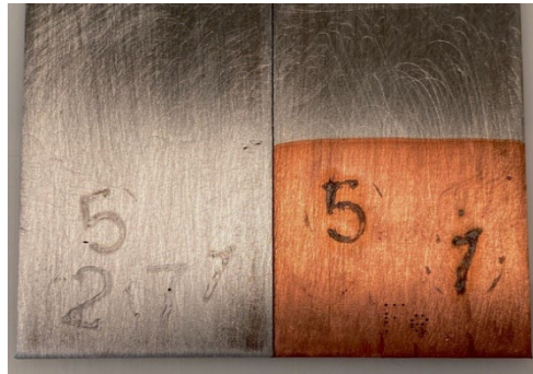
Figure 3: The electrochemical deposition of copper on iron to visualize the solution numbers 5 and 1
