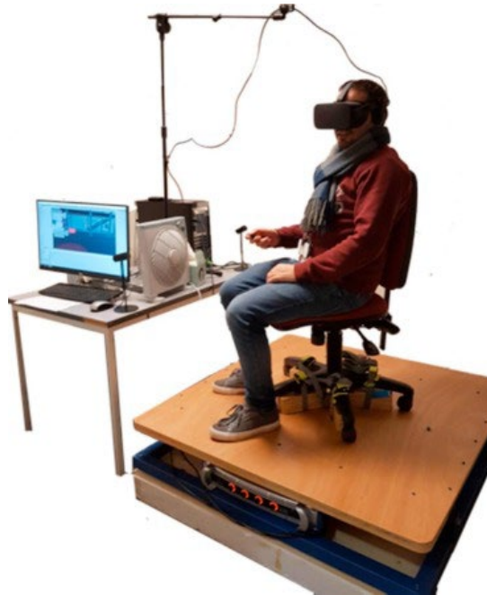
Figure 2: A tester seated on the vibrating platform. (Lovreglio et al., 2018)
