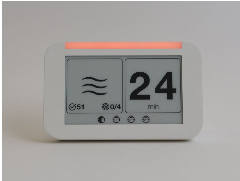
Figure 1: Photograph of the ASA showing the E-ink display with a running Pomodoro countdown. The visible red light signals to others that the learner has begun a focused interval and should not be interrupted
