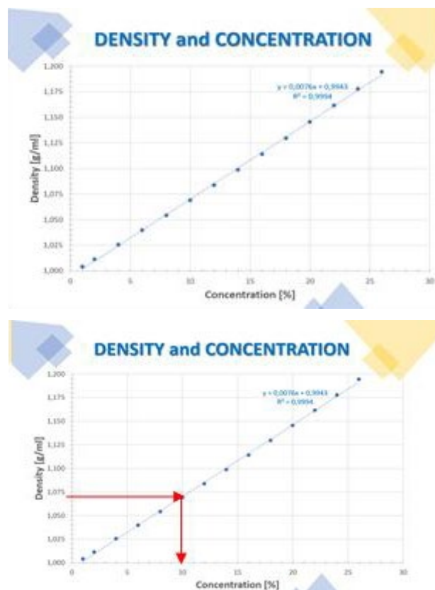
Figure 8: Diagram for density and concentration of sodium chloride solutions. Left as they find it, right how to read the result
