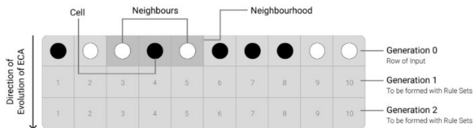
Figure 1: Abstraction of ECA Structure
