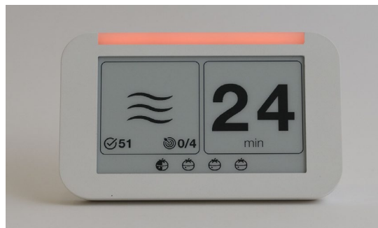
Figure 1: The ASA interface during a focus interval: state panel (left), countdown panel (right), daily-goal tomato row (bottom), red status light (top)
