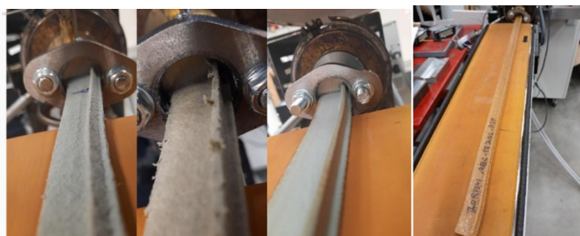
Figure 2: Left: Variation of the surface quality of biocomposite samples (Image: Reijo Heikkinen). Right: A lab-scale extruder producing a biocomposite profile. (Image: Kusti Ruokamo)
