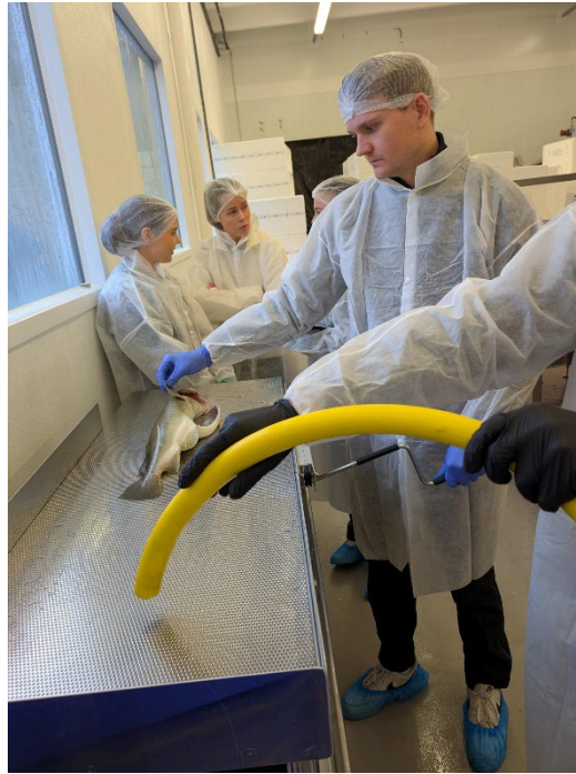
Figure 2: First friction jig test with farmed cod at processing facility
