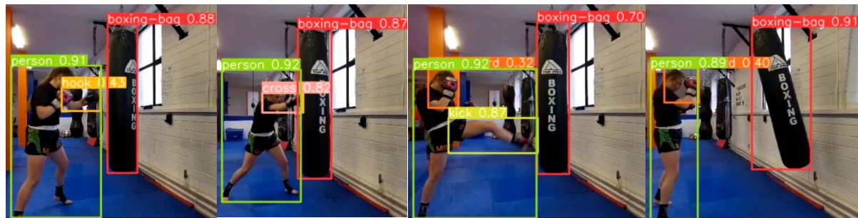
Figure 5: YOLOv8 Results from Video Sample - Hook, Cross, Kick, High Guard, Person, and Boxing-Bag Classes
