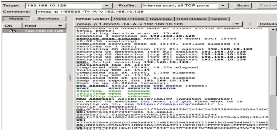
Figure 3: Nmap scanning for all open TCP ports
