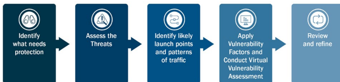
Figure 1: UAS Vulnerability Assessment Process- (U.S. Department of Homeland Security Cybersecurity and Infrastructure Security Agency)
