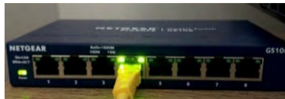
Figure 3: Port 4 is showing activity even though the uplink isn't connected (simulated as disabled)
