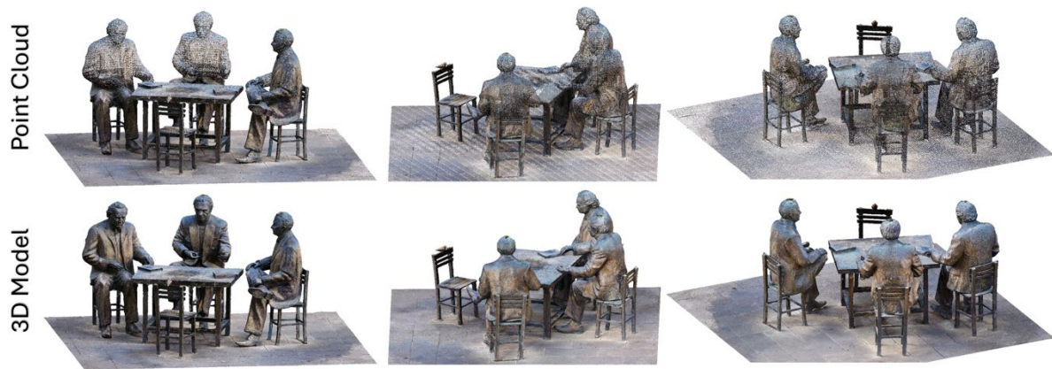
Figure 3: Point cloud (top) and textured 3D model (bottom) of the Seated Group with Table
