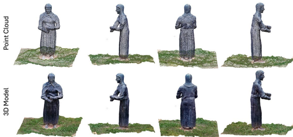
Figure 1: Point cloud (top) and textured 3D model (bottom) of the Human Statue
