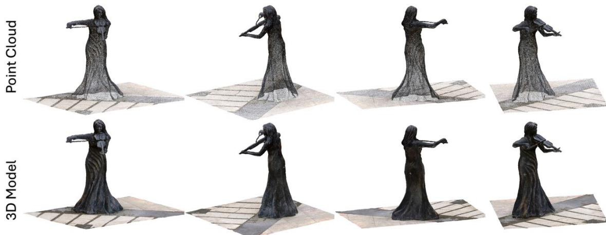
Figure 2: Point cloud (top) and textured 3D model (bottom) of the Violinist Statue
