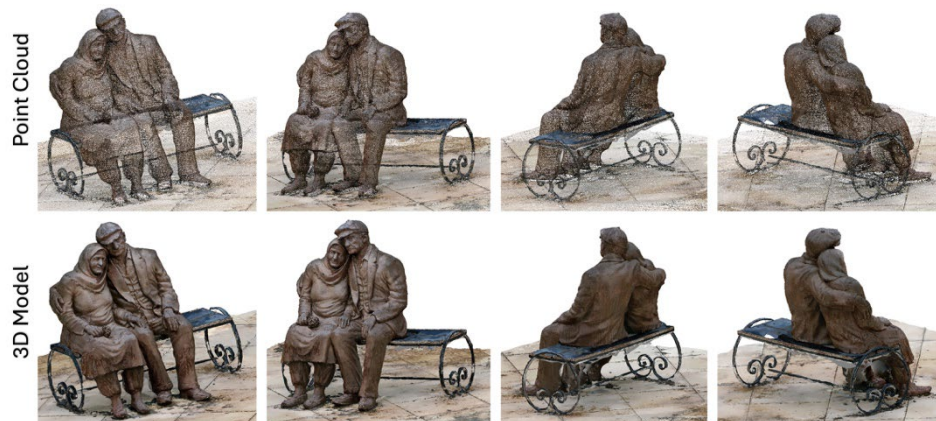
Figure 5: Point cloud (top) and textured 3D model (bottom) of the Elderly Couple on a Bench
